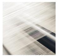
DoubleBeam<sup>2</sup> technology allows thick, 500 and 1000 denier yarns to be woven into light weight fabrics with Fiber104. The result is a fabric with outstanding strength-to-weight ratios, increased rugged durability, and multi-directional low stretch needed for shape longevity. The low stretch characteristics in all directions allow this fabric to be oriented in either a crosscut or tri-radial application, or one sail with both.
